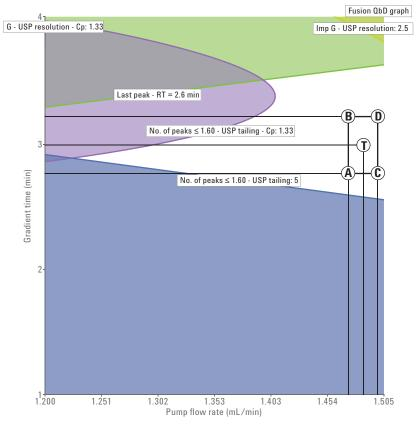
Figure 4. Final design space showing the PAR.
