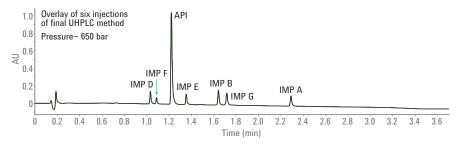
Figure 6. Reproducibility of final UHPLC method, using an overlay of six chromatograms.
