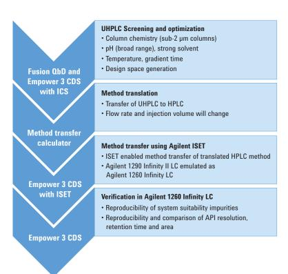
Figure 2. Overall workflow used for the study. The software packages used are shown on the left side of the flowchart, while detailed steps of the workflow are shown on the right side.
