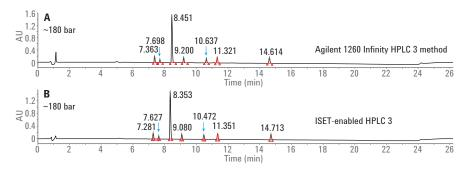
Figure 8. Overlaid chromatograms showing the similarity of ISET-emulated and an Agilent 1260 Infinity LC system for HPLC method 3.
