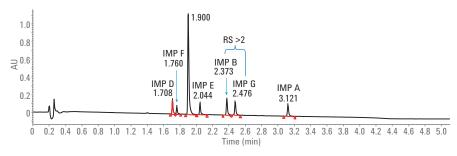
Figure 3. Resolution between impurities B and G was greater than 2, which met the ATP criteria of the screening phase.
