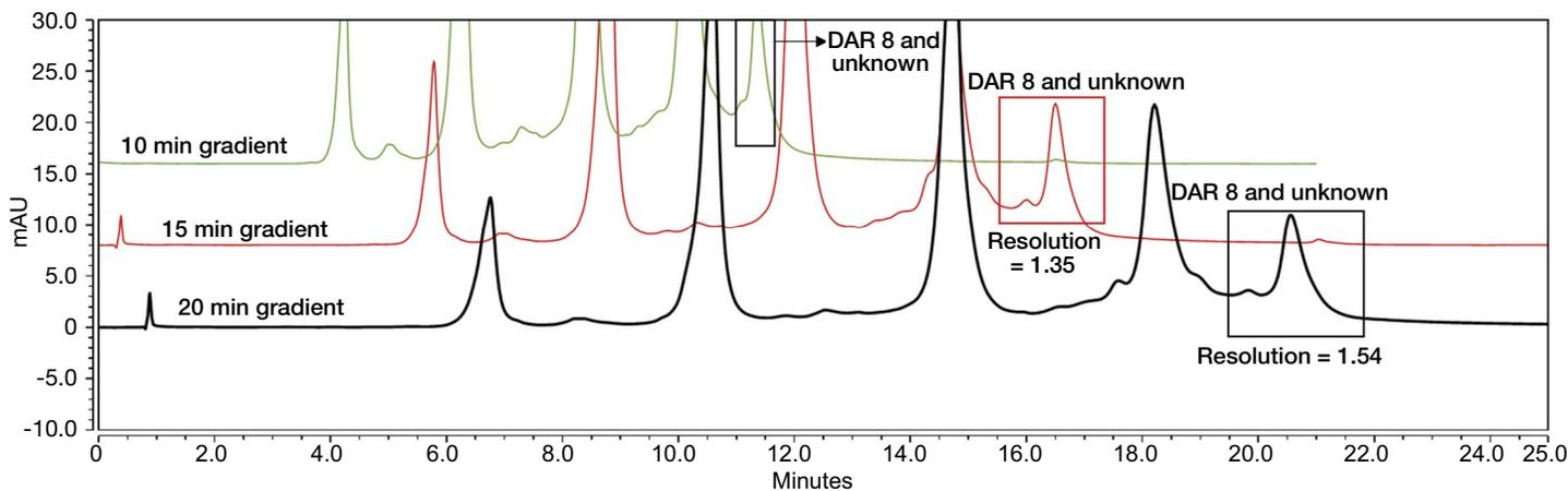
Figure 6. Separation for small unknown peaks in Brentuximab vedotin chromatograms with different gradient times
