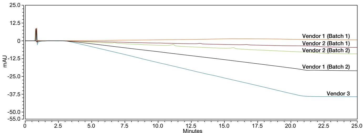
Figure 7. Chromatogram of a mixed solvent of eluent A and water (1:1, v/v) injections using ammonium sulfate from different vendors
