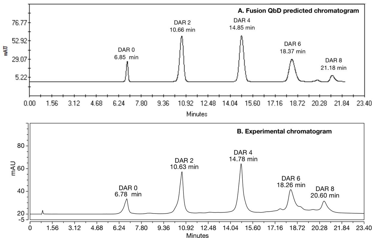
**Figure 3. Comparison of predicted (A) and experimental (B) chromatograms of brentuximab vedotin.** Fusion QbD software predicted the best conditions: Pump flow rate: 0.80 mL/min, Gradient time: 18.5 min, Initial % eluent B: 5.0%, Column temp.: 25.0 °C.
