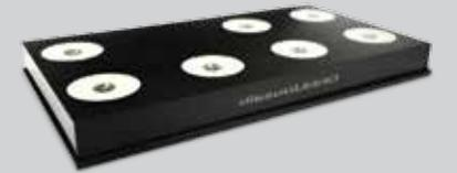
evaluate physical parameters such as centering, wobble and paddle rotation speed. dissoGUARD® can be retrofitted to any Agilent 708-DS or 709-DS apparatus. To learn more about this system, visit [www.dissoguard.com](http://www.dissoguard.com).
